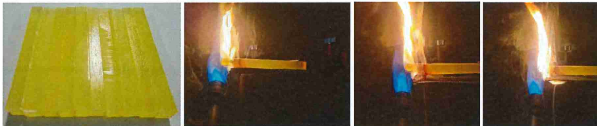
Figs. 2a – 2d: Sample ‘fingers’ before and during testing
