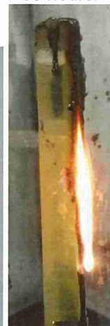
Figs. 5a & 5b: Sample 'fingers' before and during testing
